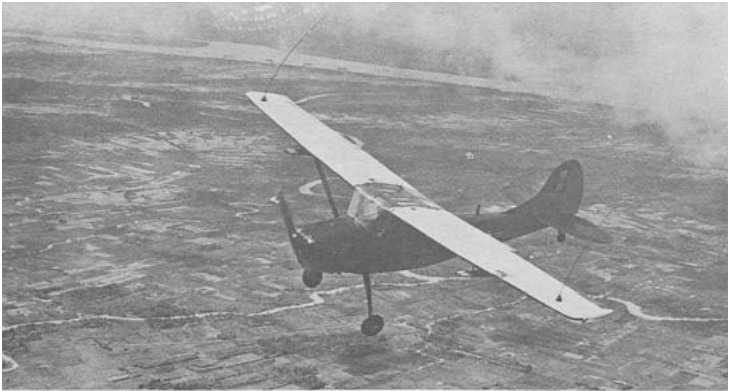
South Vietnamese O-1 "Bird Dog" used for observation and forward air control
